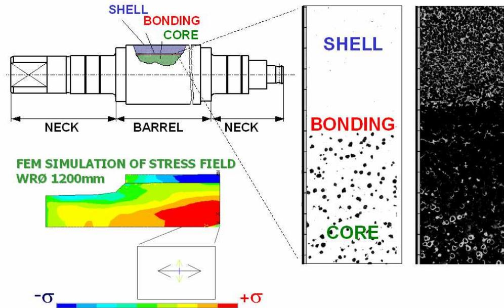
**Figure 2: principle of compound rolls [1]**
