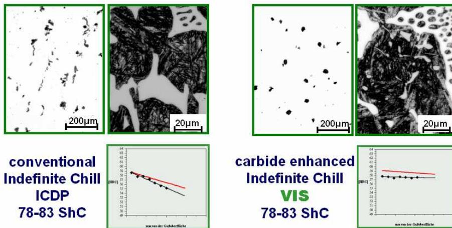
Figure 10: comparison of shell microstructure and hardness drop of conventional ICDP and carbide enhanced Indefinite (VIS) [6]
